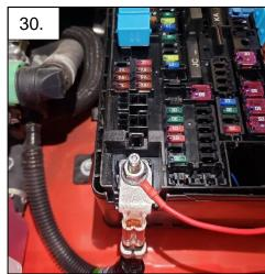
31. Using a 10mm socket, remove the common ground bolt that the main harness relay is secured to and install the negative (black) ring terminal. Replace the ground bolt. Plug the S8 into the wiring harness and test the light.
